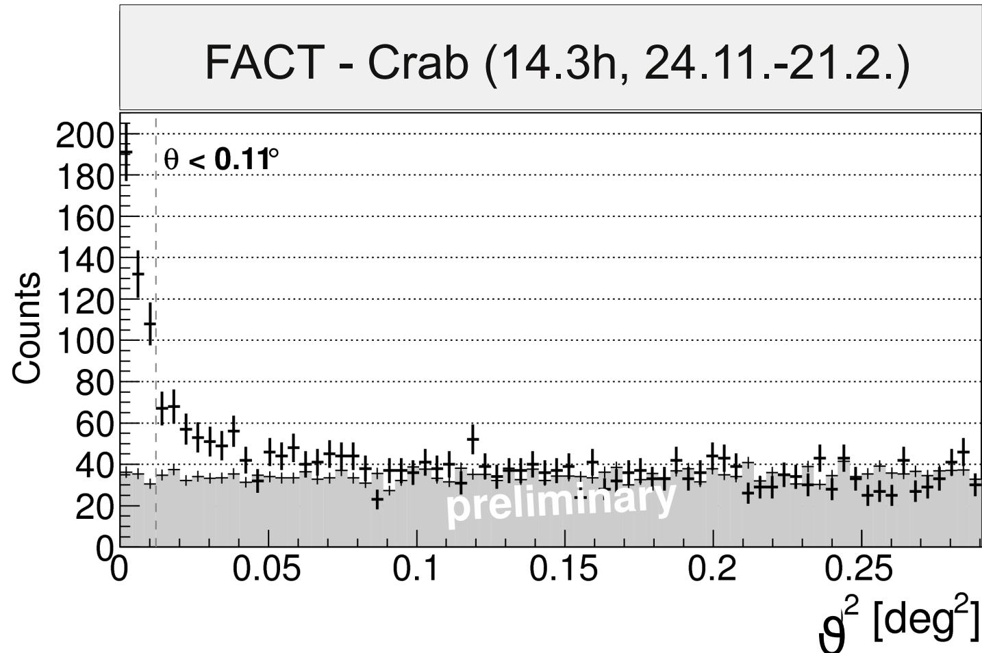
Angle between reconstructed shower origin and target position
