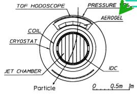
Figure 1: BESS spectrometer
